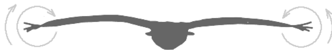
Figure 13. View on a flying goose and the upwash left and right of it.
